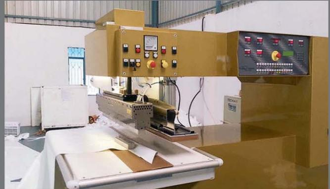
High-temperature PTFE (Polytetrafluoroethylene) heat sealing machine to weld fabric membranes.
