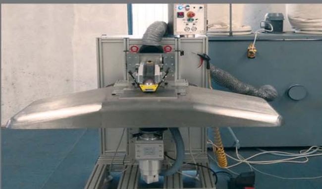
Abrasion machine for grinding special non-weldable for fabrics. Made in Italy
